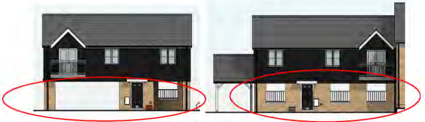
Images 15a – 15b. Typical FOG unit, comprising a flat above car parking, or a flat above a parking courtyard access.
