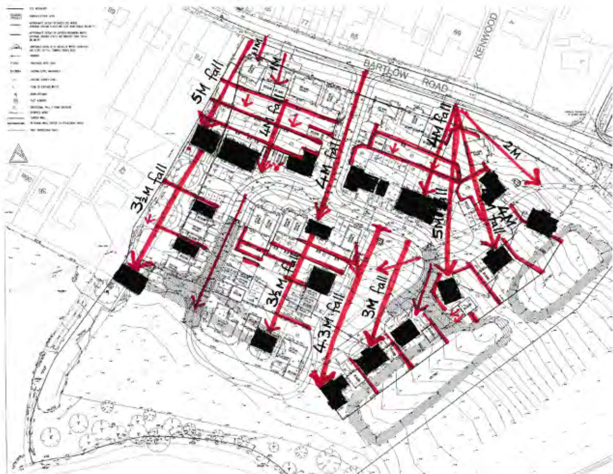
Image 7. South Site terracing, levels and slopes down the proposed development. The Levels Plan used as a base shows the three unauthorised mounds within the proposed scheme.
