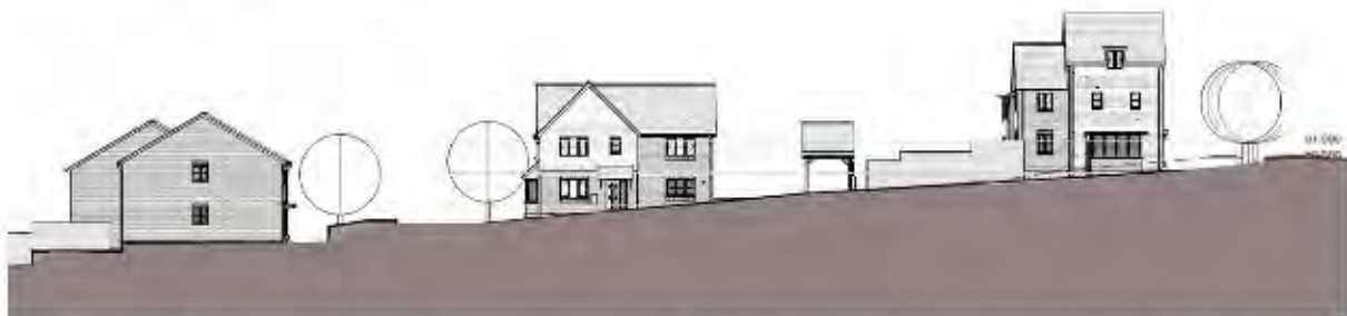
Image 23. Site Section 4. Note Bartlow Road is at 49.800 (so higher) according to the Levels Plan.
